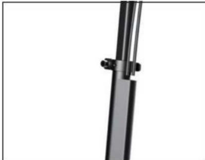
Step 4: unscrew the nut.
