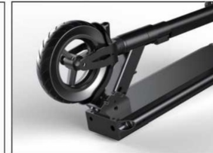
Step 6: push forward and at the same time hold down the lever when folding the head.
