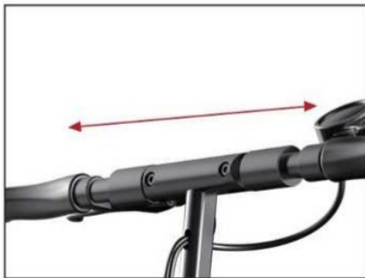
Step 2: extend the T-shaped sleeve outward
