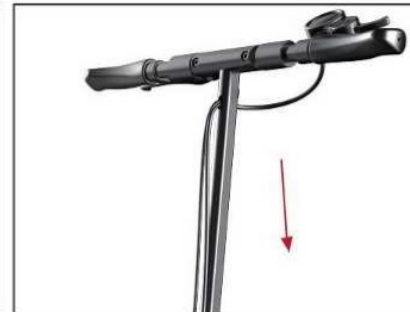
Step 5: adjust T-shaped tube downward
