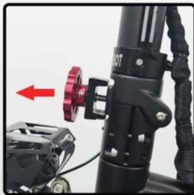
② Keep loosening the folding knob until the T-shaped buckle completely leaves the grooves
